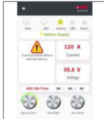
COMMUNICATION FAILURE BETWEEN BATTERY AND POWER SOURCE
