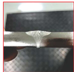
8+8 mm Cr-Ni Full Penetration weld
