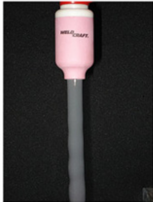
This photo shows the even gas flow created by using a gas lens.
