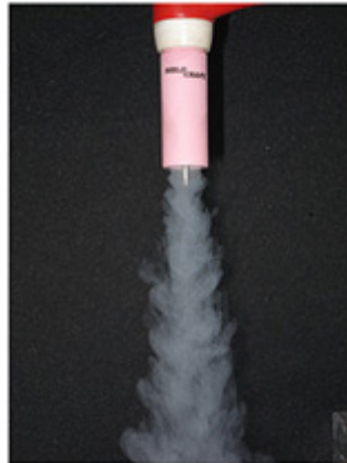
Photo shows gas coverage without a gas lens.
