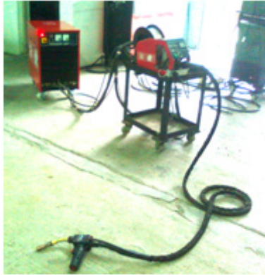
Typical setup of GMAW process for Aluminum welding with Pushpull Torch.
