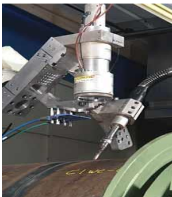
Fig.4a. Nd: YAG laser - MAG hybrid process being developed for land pipeline girth welding. Picture of the welding head
