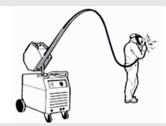
Special attachments and extensions to interconnection cables reduce welder fatigue for welding at long distances from the Power Source
