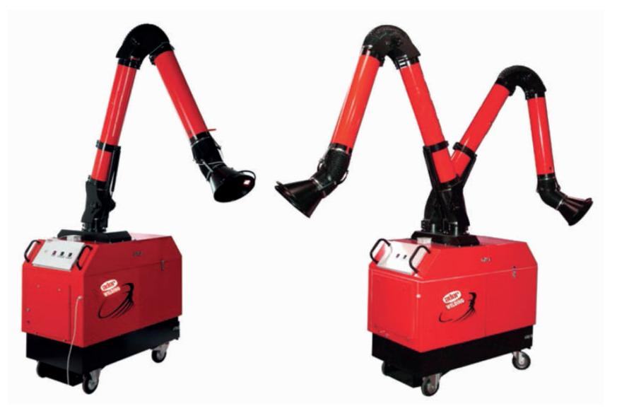
Welding areas require adequate ventilation and local exhaust to keep fumes and gases from the breathing zone and the general area.
