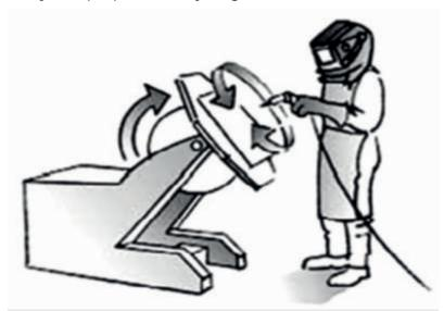
Rotators are used to rotate a job with circular or cylindrical profile to help the welder consistently without changing his position and welding torch angle continuously
