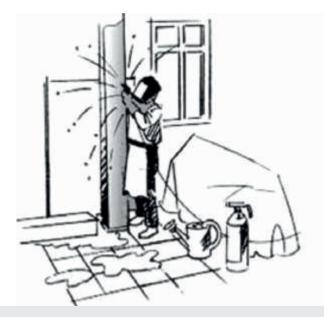
It is important to protect fire-sensitive things where there is a risk of fire during welding. Fire extinguishers with foam - spray system and buckets filled with sand must be placed adjacent to all welding zones
