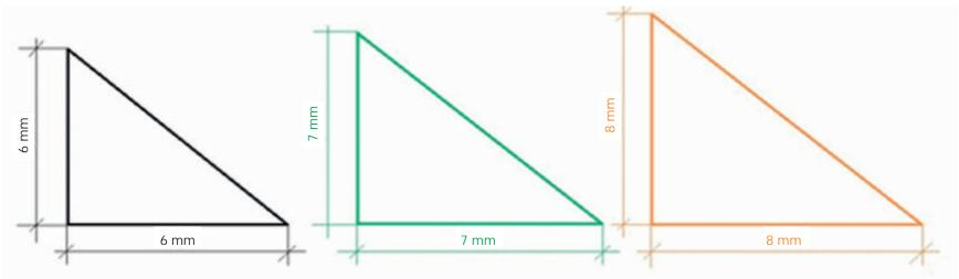
The actual size of the Fillet specified as per the drawings is 6 mm.
