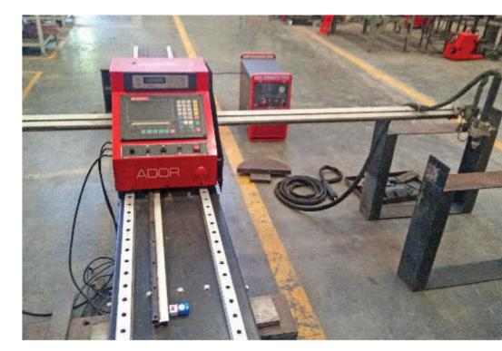
A small CNC cutting machine for smaller plate sizes Portable CNC flame and plasma cutting machine-King Cut Smarty from Ador Welding
