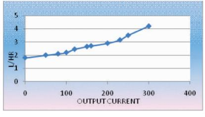
No load fuel consumption is less i.e 1.8 L/Hr, hence less fuel consumption during no-load condition which means more profit to customer.
