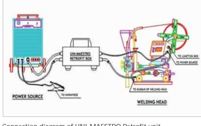
Connection diagram of UNI-MAESTRO Retrofit unit with SAW power source:
