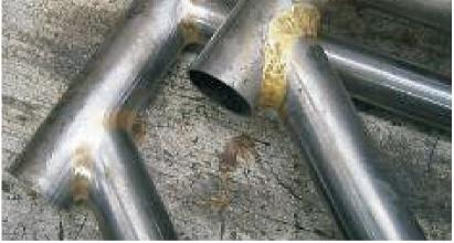
When using Bracc 2211, melt the flux from end of the rod on to the start of the weld area. Continue heating the weld area until the flux melts. Next melt a drop of filler metal by playing with the flame on the rod end until it flows and bonds easily. Continue adding more of the filler metal drop by drop into the joint.
