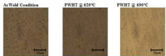
Fig 3.2 308L - FN7 weld metal microstructure with different PWHT temperature
