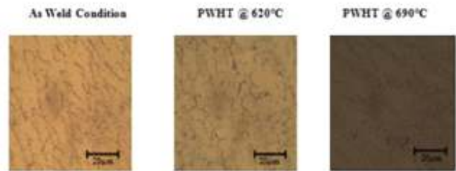
Fig 3.1 308L - FN4 weld metal microstructure with different PWHT temperature
