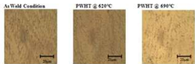
Fig 3.3 308L - FN11 weld metal microstructure with different PWHT temperature
