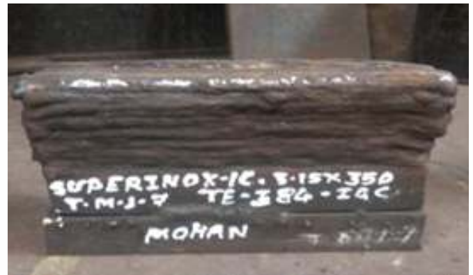
Fig 2.3 Prepared IGC weld pad
