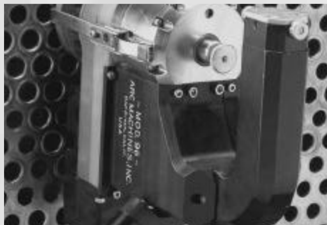
Tube to Tube-Sheet Welding
