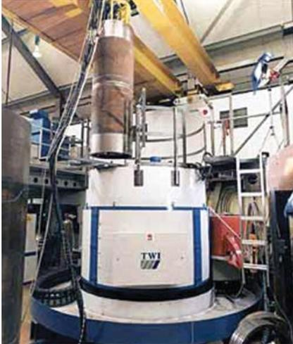
more conventional pressure for EB welding of  $5 \times 10^{-3}$  mbar. This reduced pressure option does away with the need for large vacuum chambers and worries about leaks and seals. Simple mechanical pumps and local seals are sufficient to achieve  $\sim 1$  mbar. These systems are also more tolerant to fluctuations in working vacuum pressure, gun to work distance and work-piece cleanliness.
