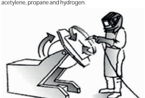
Rotators are used to rotate a job with circular or cylindrical profile to help the welder consistently without changing his position and welding torch angle continuously
