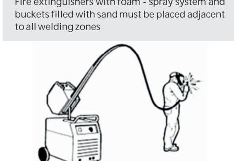
Special attachments and extensions to interconnection cables reduce welder fatigue for welding at long distances from the Power Source
