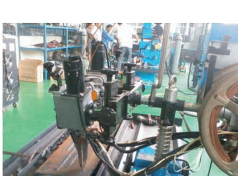
The Figure above shows Tandem Twin Submerged Arc Welding
