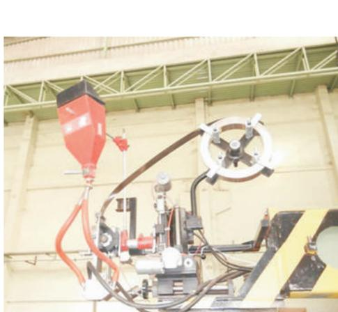
All of the above are variations of the standard submerged arc welding processes that give increased productivity by using higher welding currents and current densities. However, before selecting a variation, it is necessary to consider other factors, such as material thickness, production level, batch size, throughput requirements, joint preparation, and code quality.
