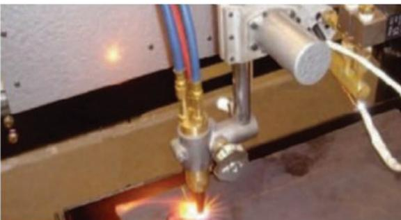
Motorized torch lifter allows torch adjustment from controller
