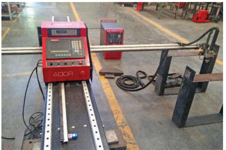
A small CNC cutting machine for smaller plate sizes
