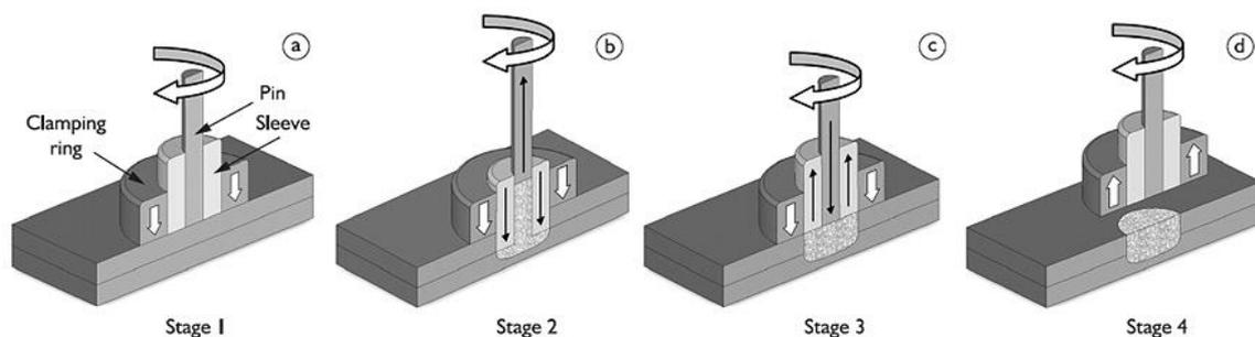
Fig. Working principle of friction spot welding
