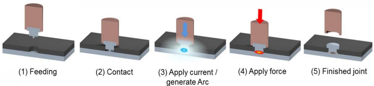
Fig. Process principle of arc element welding with an auxiliary joining part
